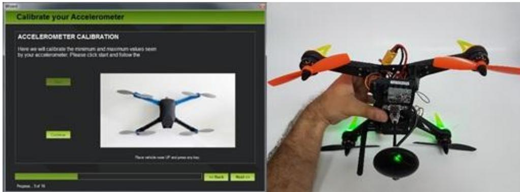
Place the drone tilting or 180 forward as shown in the picture below and press "Continue".
